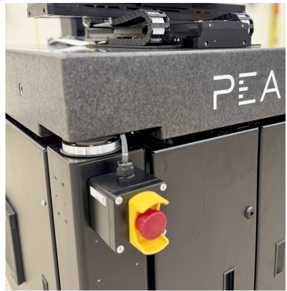
Emergency Stop button
