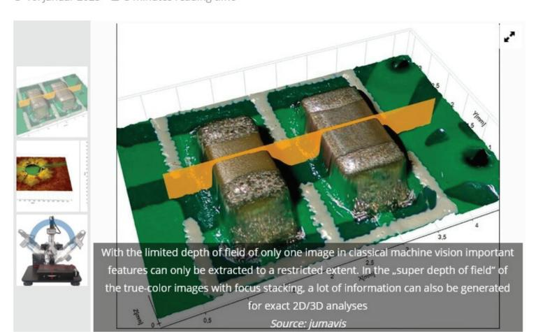
Super depth of field through focus stacking (up to 250 focus positions combined to a 2D/3D image) provides a very extensive expansion of analysis options compared to classic 2D machine vision (one image plane with one depth of field).
