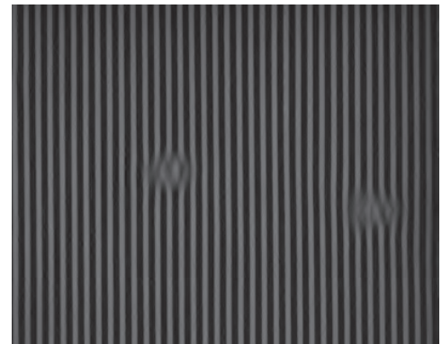
Seal inspection with BL44-660 (red) light with distortion diffuser.
