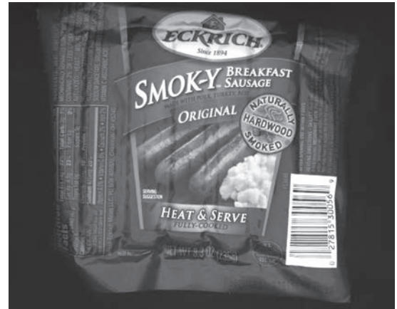
Washdown dome removes glare from product
