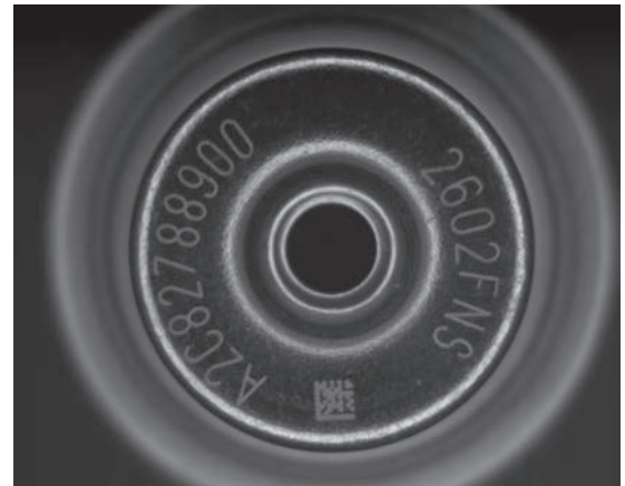
Part inspection with OL66-WHI
