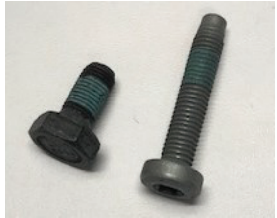
Bolts with Resin Coating Applied.
